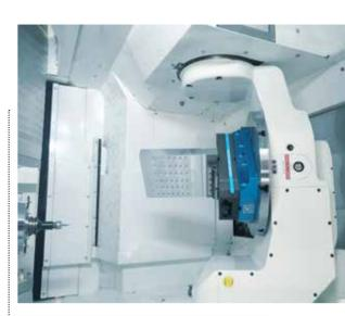
the range offer, especially oriented to the production of driven tool-holders for NC turning centres, which allow executing milling, drilling and tapping operations on the lathe itself without further setups.
